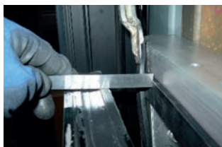
Displacement dZ : IGU before pushing onto the curved sub-construction
