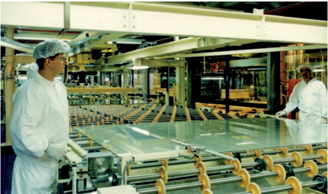
Production of laminated safety glass – clean room
