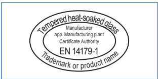
Identification of tempered heat-soaked glass
