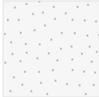
Bird1st Etch SqX22 THREAT FACTOR: 20 Non-directional 6mm squares, randomly spaced no more than 2" x 2" apart
