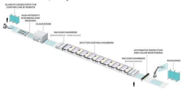
**Figure 3 - Vacuum Sputter Coating Process**
