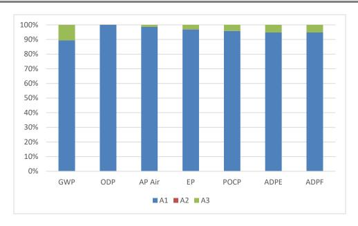
Figure 4 - Relative Contributions of Cradle to Gate Life Cycle Stages for Sputter Coated Glass
